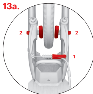
13a. Adjusting the rear brake (V-brake)
