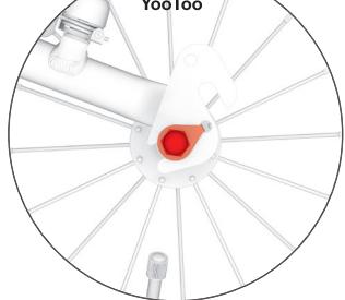
The lower dropout, on the contrary, enables the seat to be positioned higher than usual. **Warning:** after each position change, readjust the brakes.
