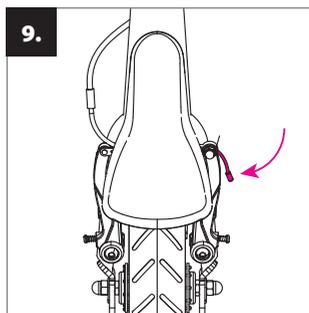
Bend the ending of the brake cable so that it does not obstruct when the child is riding.
